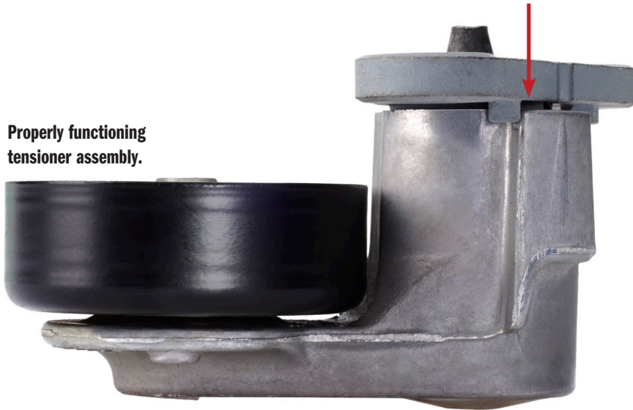
Tensioner stop with normal operation of tensioner.
